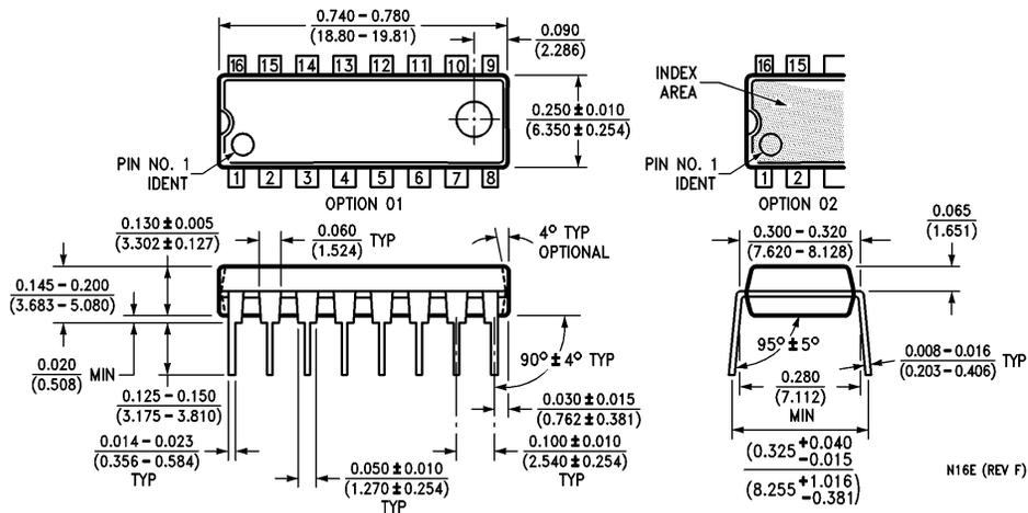
**16-Lead Molded Dual-In-Line Package (N)**
