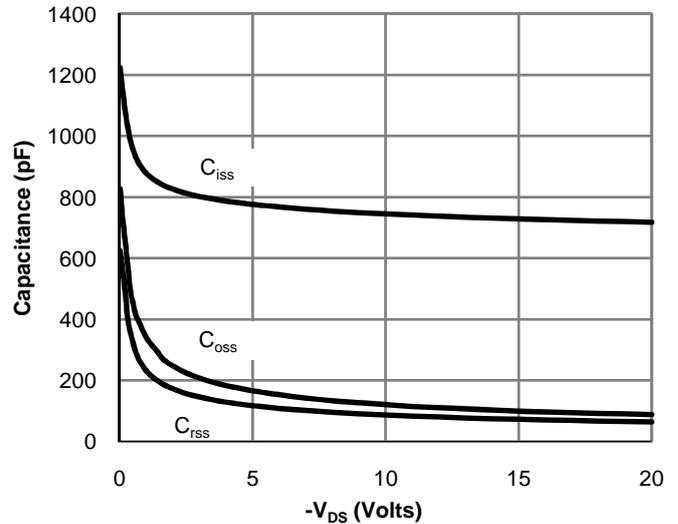
Figure 8: Capacitance Characteristics
