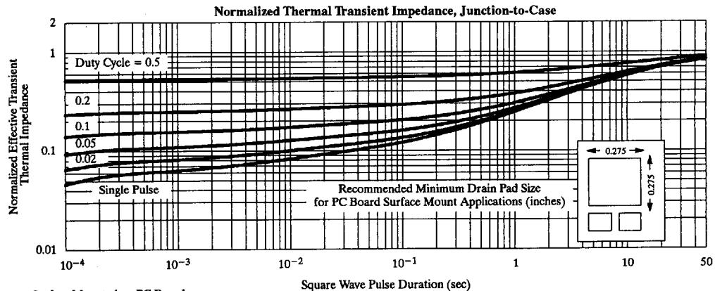
a. Surface Mounted on PC Board.
