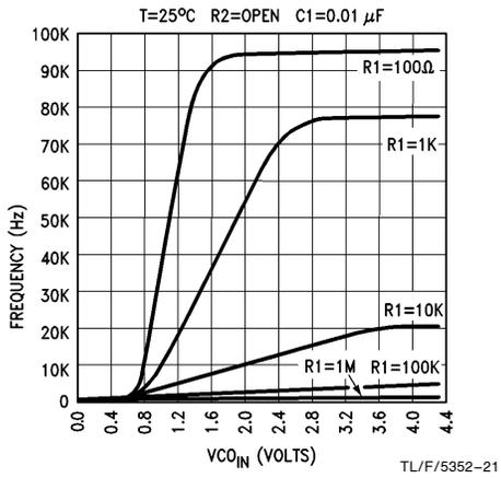
**HC4046 VCO<sub>in</sub> vs f<sub>out</sub> V<sub>CC</sub> = 4.5V**
