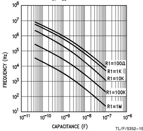
**Typical Center Frequency vs R1, C1**  $V_{CC} = 6V$
