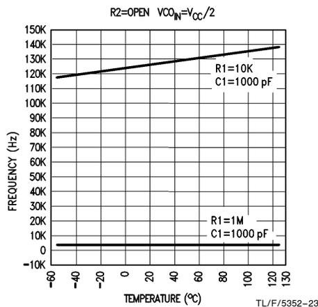
**HC4046 VCO<sub>out</sub> vs Temperature V<sub>CC</sub> = 6V**
